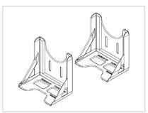
Designed to be taped to the insulated glass inside a Contemporary Hybrid aluminum frame and guides the Accent into place for perfect positioning and quick installation. Reusable.
